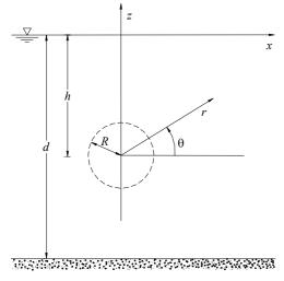
Figure 7. Froude-Krylov force on a horizontal submerged cylinder: the reference frame.
