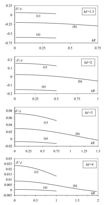
Figure 8. Horizontal component of the Froude-Krylov force on a horizontal submerged cylinder. The parameter  $\delta/\varepsilon$  as function of kR, for fixed values of kd: (a) h/d = 0.25; (b) h/d = 0.50; (c) h/d = 0.75
