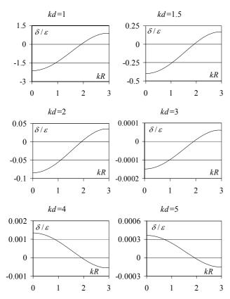
Figure 6. Froude-Krylov force on a vertical cylinder: the parameter  $\delta/\varepsilon$  as function of kR, for fixed values of kd.
