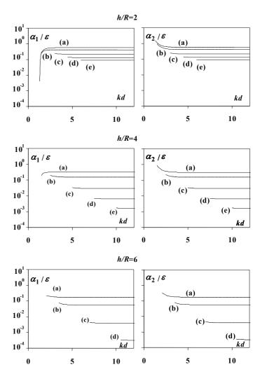
Figure 9. Vertical component of the Froude-Krylov force on a horizontal submerged cylinder: the parameters  $\alpha_1/\varepsilon$  and  $\alpha_2/\varepsilon$  as function of kd, for fixed values of h/R.
